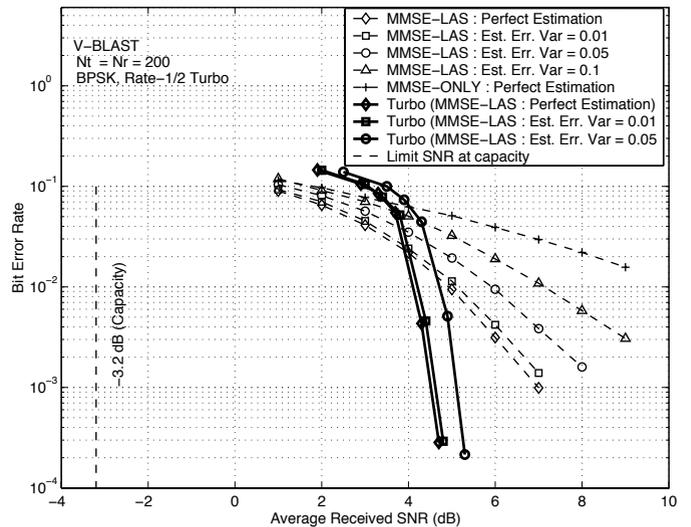
Fig. 9. Effect of channel estimation errors on uncoded and coded BER performance of the proposed MMSE-LAS detector in a  $200 \times 200$  V-BLAST system with BPSK and rate-1/2 turbo code. Channel estimation error variance,  $\sigma_e^2 = 0, 0.01, 0.05, 0.1$ .
