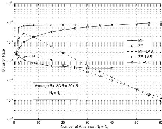
Fig. 1. Uncoded BER performance of MF/ZF-LAS detectors as a function of number of transmit/receive antennas ( $N_t = N_r$ ) for V-BLAST at an average received SNR = 20 dB. BPSK,  $N_t$  bps/Hz spectral efficiency.
