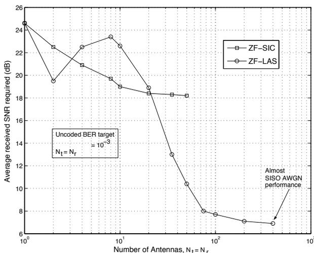
Fig. 4. Average received SNR required to achieve a target uncoded BER of  $10^{-3}$  in V-BLAST for increasing values of  $N_t = N_r$ . BPSK. ZF-LAS versus ZF-SIC. ZF-LAS achieves near SISO AWGN performance.
