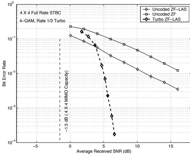
Fig. 11. Uncoded and coded BER performance of ZF-LAS for a  $4 \times 4$  full-rate (i.e., rate-4) non-orthogonal STBC from Division Algebras given in (21). 4-QAM, rate-1/3 turbo code. 8/3 bps/Hz spectral efficiency.
