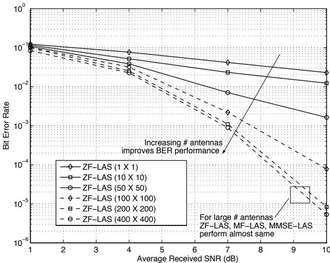
Fig. 3. Uncoded BER performance of ZF-LAS for V-BLAST as a function of average received SNR for increasing values of  $N_t = N_r$ . BPSK,  $N_t$  bps/Hz spectral efficiency. For large number of antennas (e.g.,  $N_t = N_r = 200, 400$ ), the performance of ZF-LAS, MF-LAS, and MMSE-LAS are almost the same.
