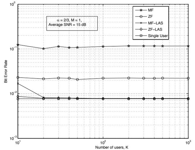
Fig. 13. BER performance of ZF-LAS and MF-LAS detectors as a function of number of users,  $K$ , for single carrier CDMA ( $M = 1$ ) in Rayleigh fading for a fixed  $\alpha = 2/3$  and average SNR = 15 dB.  $N$  varied from 15 to 1500.
