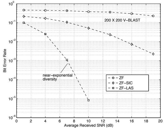
Fig. 2. Uncoded BER performance of ZF-LAS versus ZF-SIC as a function of average received SNR for a  $200 \times 200$  V-BLAST system. BPSK, 200 bps/Hz spectral efficiency. ZF-LAS achieves higher order diversity (near-exponential diversity) than ZF-SIC at a much lesser complexity.
