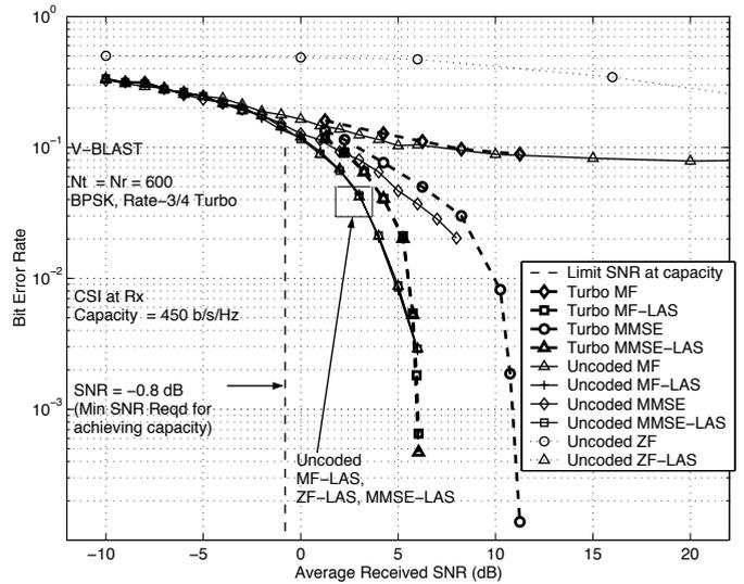
Fig. 8. BER performance of various detectors for rate-3/4 turbo-encoded data using BPSK symbols in a  $600 \times 600$  V-BLAST system. 450 bps/Hz spectral efficiency. Proposed MF/ZF/MMSE-LAS detectors' performance is away from capacity by 7 dB.
