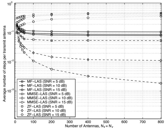
Fig. 5. Complexity of the LAS algorithm in terms of average number of steps per transmit antenna till fixed point is reached in V-BLAST as a function of  $N_t = N_r$  for different SNRs and initial vectors (MF, ZF, MMSE). BPSK. Results obtained from simulations.
