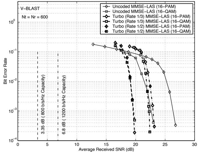
Fig. 10. Uncoded and coded BER performance of MMSE-LAS in a  $600 \times 600$  V-BLAST system for 16-PAM and 16-QAM with rate-1/2 and rate-1/3 turbo codes.
