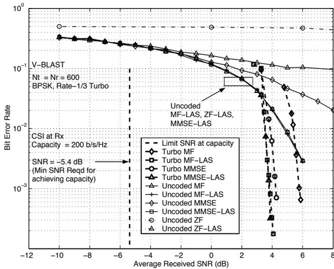
Fig. 7. BER performance of various detectors for rate-1/3 turbo-encoded data using BPSK symbols in a  $600 \times 600$  V-BLAST system. 200 bps/Hz spectral efficiency. Proposed MF/ZF/MMSE-LAS detectors' performance is away from capacity by 9.4 dB.
