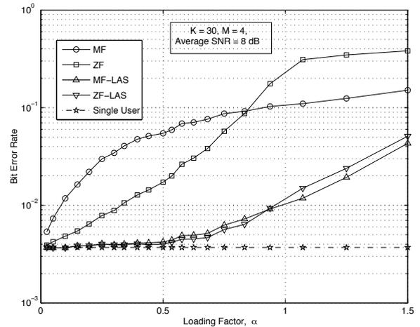
Fig. 15. BER performance of ZF-LAS and MF-LAS detectors as a function of loading factor,  $\alpha$ , for multicarrier CDMA in Rayleigh fading.  $M = 4$ ,  $K = 30$ ,  $N$  varied from 300 to 5, average SNR = 8 dB.
