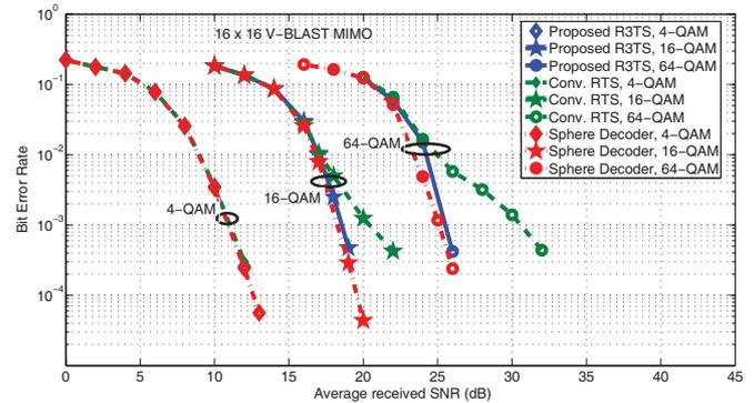
Fig. 1. BER performance of the proposed R3TS algorithm in comparison with those of conventional RTS algorithm and sphere decoder for  $16 \times 16$  V-BLAST MIMO with 4-, 16- and 64 QAM.
