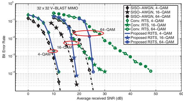
Fig. 2. BER performance of R3TS in comparison with those of conventional RTS and ML lower bound (i.e., unfaded SISO AWGN performance) for  $32 \times 32$  V-BLAST MIMO with 4-, 16- and 64 QAM.
