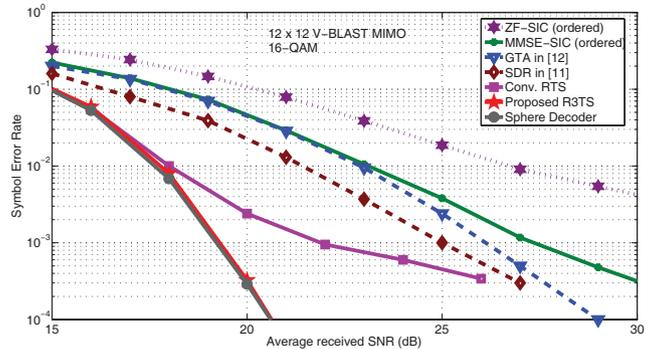
Fig. 4. SER performance comparison of R3TS algorithm with other detectors for  $12 \times 12$  V-BLAST MIMO with 16-QAM.
