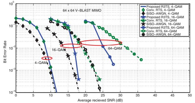
Fig. 3. BER performance of R3TS in comparison with those of conventional RTS and ML lower bound for  $64 \times 64$  V-BLAST MIMO with 4-, 16- and 64 QAM.
