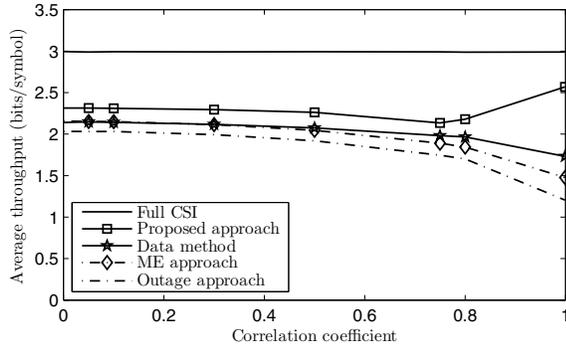
Fig. 3. Greedy scheduler: Throughput as a function of correlation coefficient  $\rho$  for different approaches ( $K = 10$ ,  $N = 10$ , and  $\bar{\gamma}_k = 9$  dB,  $1 \leq k \leq K$ ).
