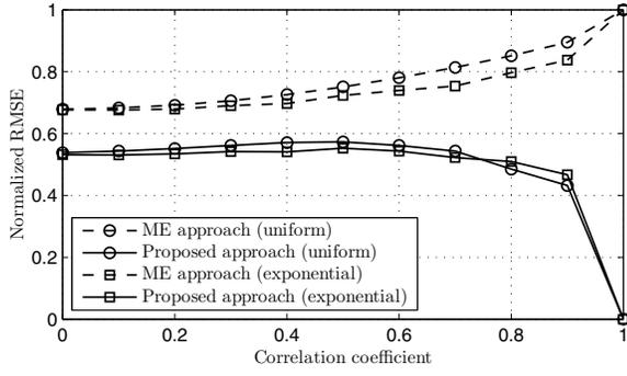
Fig. 2. Normalized RMSE (RMSE/ $\bar{\gamma}$ ) as a function of correlation coefficient  $\rho$  for ME and proposed approaches ( $N = 4$ ).
