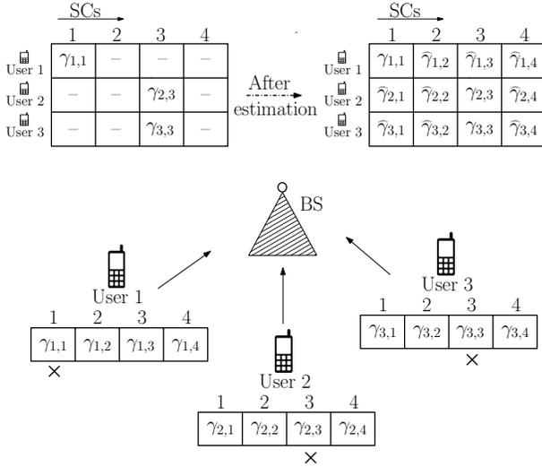
Fig. 1. Illustration of best- $m$  feedback by 3 users and scheduling at the BS ( $N = 4$  and  $m = 1$ ). Cross marks (X) denote the SCs that are fed back.
