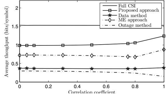
Fig. 4. RR scheduler: Throughput as a function of correlation coefficient  $\rho$  for different estimators ( $K = 10$ ,  $N = 10$ , and  $\bar{\gamma}_k = 9$  dB,  $1 \leq k \leq K$ ).
