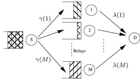
Fig. 1. Schematic of a two-hop queued cooperative relay network
