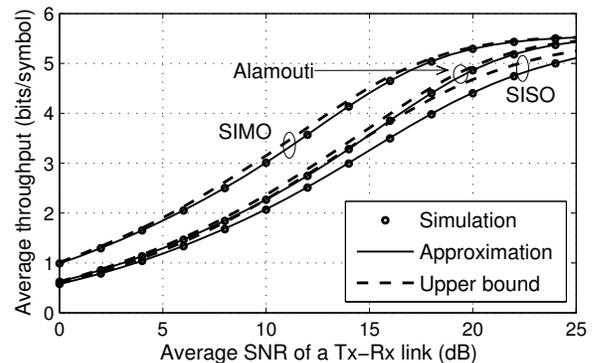
Fig. 5. LTE: Average throughput versus average SNR of a transmit-receive antenna pair link ( $\sigma^2$ ) for the TU channel.
