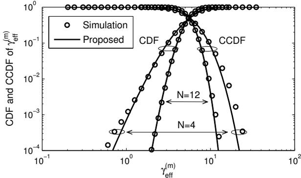
Fig. 1. Comparison of CDF and CCDF of EESM with the proposed Beta model for independent subcarriers ( $\tau = 2$  (SISO),  $\sigma^2 = 10$  dB, and  $\beta_m = 5$ ).
