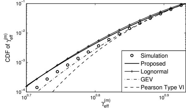
Fig. 3. Comparison of CDFs of different approximations with the empirical CDF for geometrically correlated subcarriers ( $\tau = 4$  ( $1 \times 2$  SIMO),  $\sigma^2 = 10$  dB,  $\beta_m = 5$ ,  $N = 12$ , and  $\rho = 0.4$ ).
