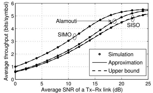
Fig. 4. LTE: Average throughput versus average SNR of a transmit-receive antenna pair link ( $\sigma^2$ ) for the RA channel.
