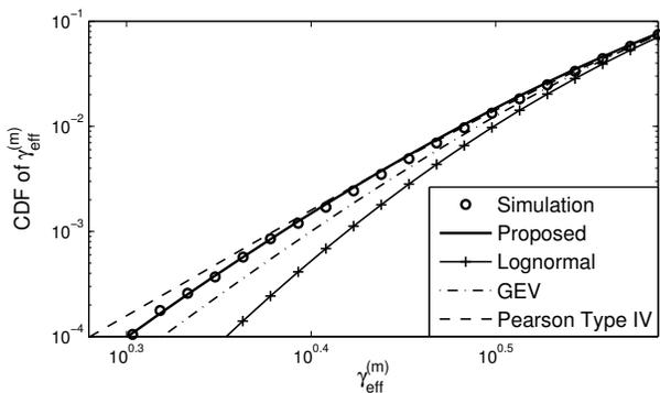
Fig. 2. Comparison of CDFs of different approximations with the empirical CDF for independent subcarriers ( $\tau = 2$  (SISO),  $\sigma^2 = 10$  dB,  $\beta_m = 5$ , and  $N = 12$ ).
