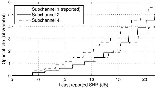
Fig. 2. Correlated subchannels: Optimal rate against the least reported SNR for different subchannels ( $N = 4$ ,  $M = 1$ , and  $\Omega = 14$  dB).
