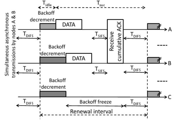
Fig. 1. Timing diagram for the proposed scheme showing a system-wide renewal interval in which two simultaneous asynchronous transmissions to the AP occur.
