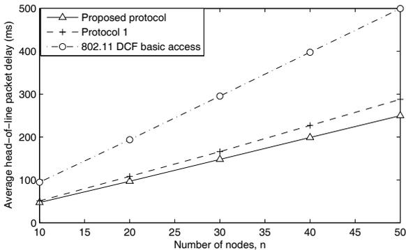
Fig. 5. Saturation delay as a function of the number of nodes
