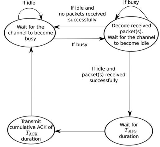
Fig. 2. Proposed protocol: Finite state machine for the access point
