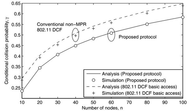
Fig. 6. Conditional packet collision probability as a function of the number of nodes
