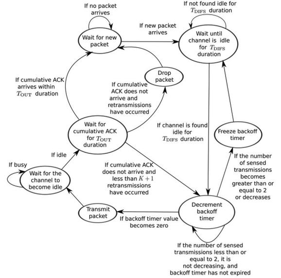
Fig. 3. Proposed protocol: Finite state machine for a node
