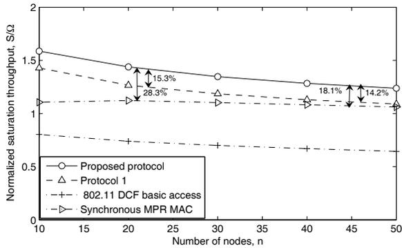
Fig. 4. Saturation throughput as a function of the number of nodes
