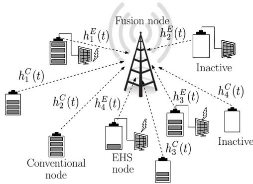
Fig. 1. A hybrid WSN consisting of  $M_E = 4$  EHS nodes and  $M_C = 4$  conventional nodes that transmit data to the FN over wireless links that undergo fading.
