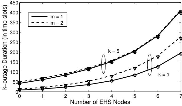
Fig. 4. Effect of  $k$  and channel fading statistics on the  $k$ -outage duration ( $M_C = 5$ ,  $\rho = 0.1$ , and  $\gamma_{th} = 1$ ). Simulation results for Nakagami- $m$  fading are shown using the markers  $\circ$  and  $\nabla$  for  $m = 1$  and  $m = 2$ , respectively.
