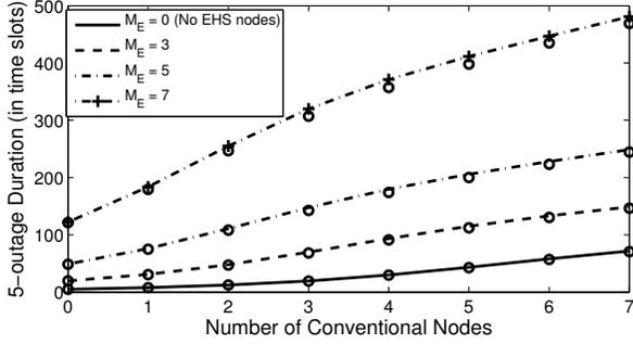
Fig. 3. Effect of  $M_E$  on 5-outage duration ( $\rho = 0.1$  and  $\gamma_{th} = 1$ ). Simulation results are shown using the marker  $\circ$ .
