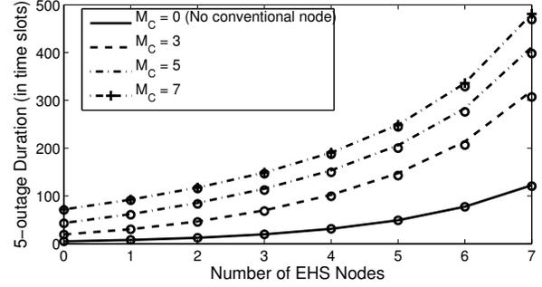
Fig. 2. Effect of  $M_C$  on 5-outage duration ( $\rho = 0.1$  and  $\gamma_{\text{th}} = 1$ ). Simulation results are shown using the marker  $\circ$ .
