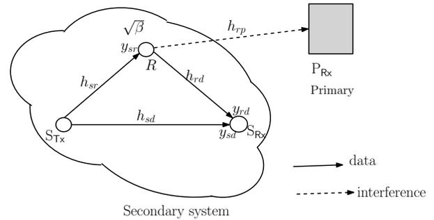
Fig. 1. Underlay CR system that consists of a secondary transmitter ( $S_{Tx}$ ) that communicates with a secondary receiver ( $S_{Rx}$ ) with the help of an AF relay in the presence of a primary receiver ( $P_{Rx}$ ).
