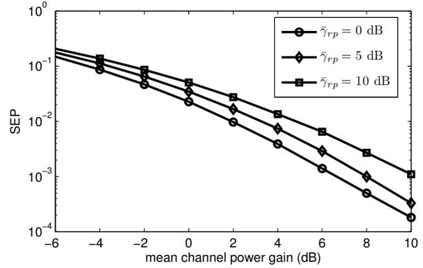
Fig. 5. Effect of R- $P_{Rx}$  link mean channel gain ( $\bar{\gamma}_{rp}$ ): SEP of ORGAP as a function of  $\gamma_{av}$  ( $\bar{\gamma}_{sr} = \bar{\gamma}_{rd} = \bar{\gamma}_{sd} \triangleq \gamma_{av}$ ,  $P_s = 15$  dB,  $I_{av} = 15$  dB, and 8PSK).
