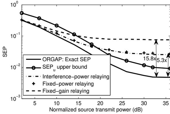
Fig. 3. Without  $S_{Tx}-S_{Rx}$  link: Comparison of SEPs of ORGAP, fixed-gain, fixed-power relaying, and interference power relaying. Also shown is the SEP upper bound ( $\bar{\gamma}_{sr} = \bar{\gamma}_{rd} = \bar{\gamma}_{rp} = 1$ ,  $I_{av} = 15$  dB, and QPSK).
