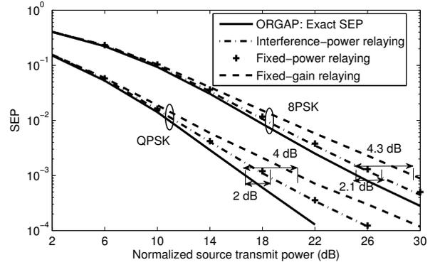
Fig. 2. With  $S_{\text{Tx}}-S_{\text{Rx}}$  link: Comparison of SEPs of ORGAP, fixed gain, and fixed-power relaying for QPSK and 8PSK ( $\bar{\gamma}_{sr} = \bar{\gamma}_{rd} = \bar{\gamma}_{rp} = \bar{\gamma}_{sd} = 1$  and  $I_{av} = 15$  dB).
