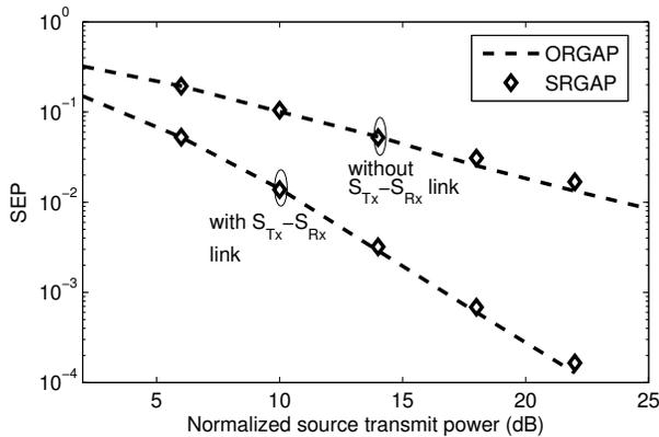
Fig. 4. ORGAP vs. SRGAP: SEP as a function of  $P_s$  ( $I_{av} = 15$  dB and QPSK).
