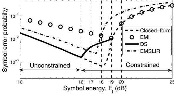
Fig. 4. Comparison of the SEPs of the closed-form optimal AS rule and several benchmark rules ( $I_{ave} = 16$  dB and QPSK).
