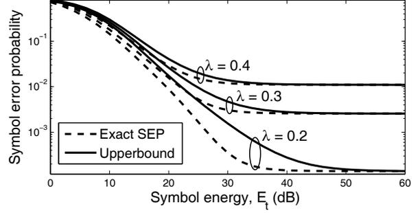
Fig. 3. SEP as a function of large  $E_t$  for different  $\lambda$  (8PSK).
