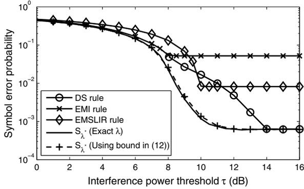
Fig. 4. SEP comparison of the optimal TAS rule and benchmark rules ( $N_t = 4$ ,  $P_t = 12$  dB,  $O_{\max} = 0.2$ ,  $c_1 = 0.5$ ,  $c_2 = 1.7$  and QPSK).
