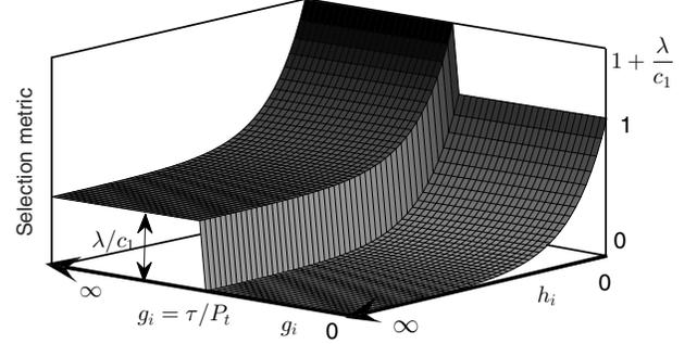
Fig. 2. Selection metric of antenna  $i$  as a function  $h_i$  and  $g_i$ .
