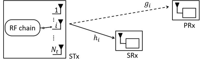
Fig. 1. System model showing a secondary system that contains an STx with  $N_t$  transmit antennas and one RF chain. It transmits data to an SRx and causes interference to a PRx.
