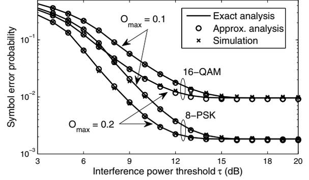
Fig. 3. SEP as a function of  $\tau$  for 8-PSK and 16-QAM for different values of  $O_{\max}$  ( $P_t = 13$  dB and  $N_t = 8$ ).
