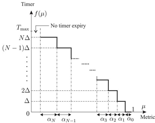
Fig. 2. Illustration of optimal metric-to-timer mapping.
