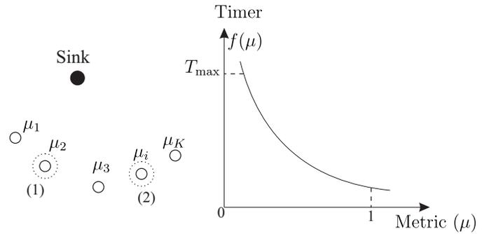
Fig. 1. A system consisting of  $K$  relays in which the best two relays need to be selected. Each relay  $i$  sets its timer depending on its metric  $\mu_i$ , and transmits a small timer packet when its timer expires.
