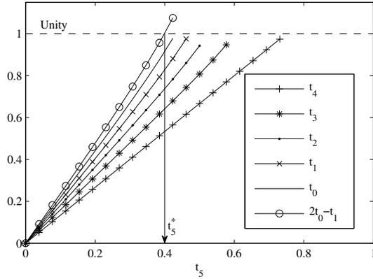
Fig. 3. Variation of  $t_i$  and  $2t_0 - t_1$  with  $t_N$  for  $K = 5$  and  $N = 5$ .
