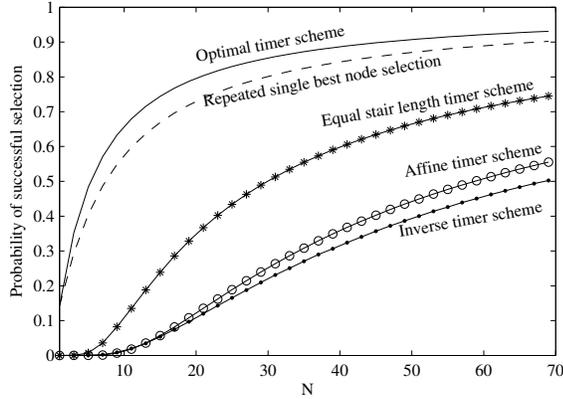
Fig. 5. Probability of selecting the best two relays out of  $K = 20$  relays as a function of the number of timer levels  $N$ .
