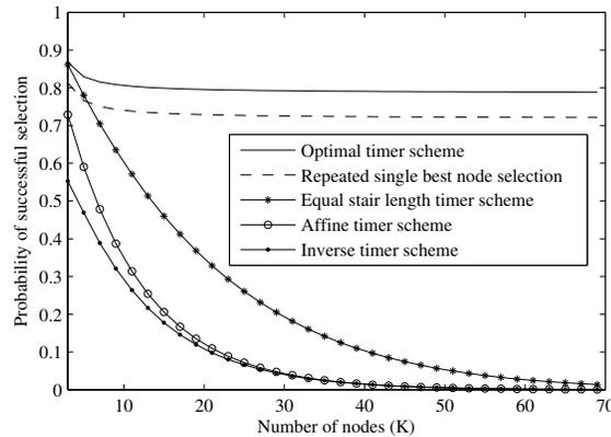
Fig. 6. Probability of selecting best two relays as a function of the number of relays in the system ( $N = 20$ ).
