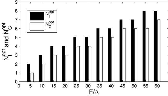
Fig. 4. Plot of optimized  $N_I$  and  $N_C$  as a function of normalized feedback overhead,  $\frac{F}{\Delta}$ , for the proposed scheme ( $K = 5$  nodes).
