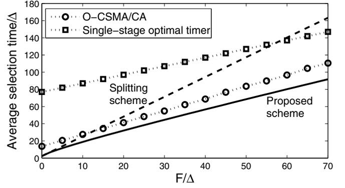
Fig. 3. Comparison of the average selection time vs. normalized feedback overhead ( $K = 5$ ). Success probability of the single-stage optimal timer is set to 98%.
