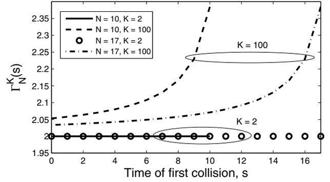
Fig. 2. Plot of the average number of nodes,  $\Gamma_N^K(s)$ , that collide at  $s\Delta$  given that the first attempted transmission was at  $s\Delta$ .
