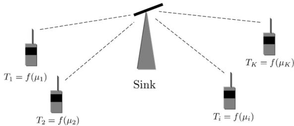
Fig. 1. A wireless system consisting of  $K$  nodes and a sink. Each node  $i$  tracks a local metric  $\mu_i$ . The sink has to select the best node with the highest metric. In the timer scheme, a node  $i$  sets its timer,  $T_i$ , as  $T_i = f(\mu_i)$ .
