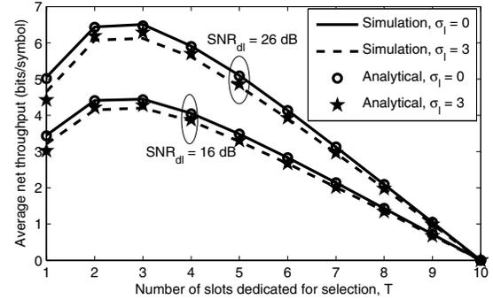
Fig. 6. Average throughput as a function of the selection duration  $T$  for different values of  $\text{SNR}_{\text{dl}}$  ( $\eta = 5$  and  $N = 25$ ).
