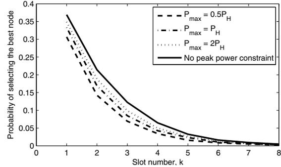
Fig. 7. Effect of peak power constraint when metric  $\mu_i$  is not coupled to  $h_i$ : Probability of selecting the best node for different values of  $P_{\text{max}}$  ( $\eta = 2$  and  $\sigma_l = 1$ ).
