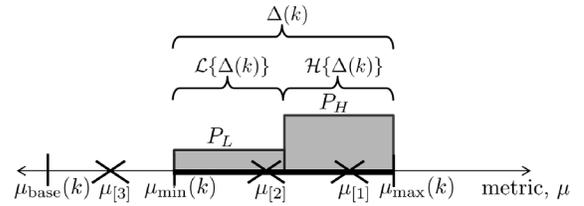
Fig. 1. Target receive powers and transmissions by different nodes based on the location of their metrics in the interval  $[\mu_{\min}(k), \mu_{\max}(k)]$ .
