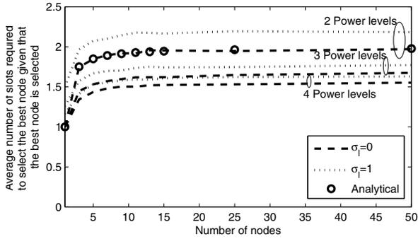
Fig. 4. Average number of slots required for selection given the best node is selected for different number of nodes  $N$  and different number of power levels  $Q$ . Analytical results for  $Q = 2$  are shown using the marker  $\circ$ .
