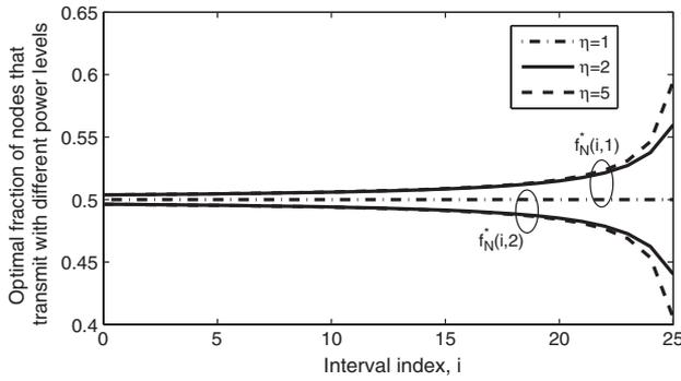
Fig. 6. Zoomed-in view of optimal fractions of nodes that transmit with different power levels for different  $\eta$  as a function of  $i$  ( $N = 25$ ,  $K = 10$ , and  $L = 2$ ).
