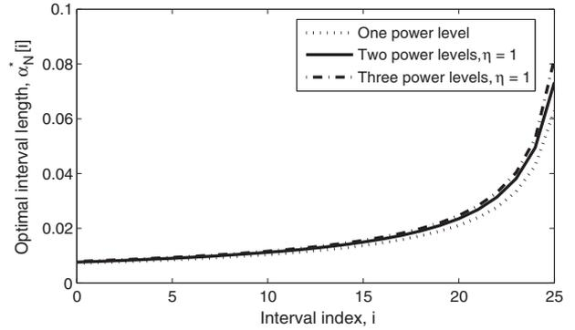
Fig. 5. Effect of number of power levels on optimal interval lengths:  $\alpha_N^*[i]$  as a function of  $i$  ( $N = 25$  and  $K = 10$ ).
