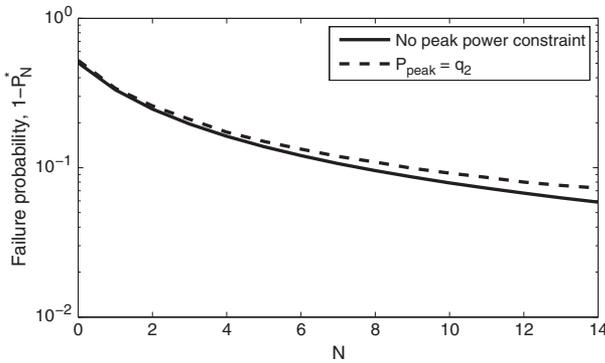
Fig. 7. Effect of peak power constraint: Zoomed-in view of failure probability:  $1 - P_N^*$  as a function of  $N$  for different peak powers when the metric of a node is its channel power gain ( $\eta = 1$ ,  $K = 10$ , and  $L = 2$ ).
