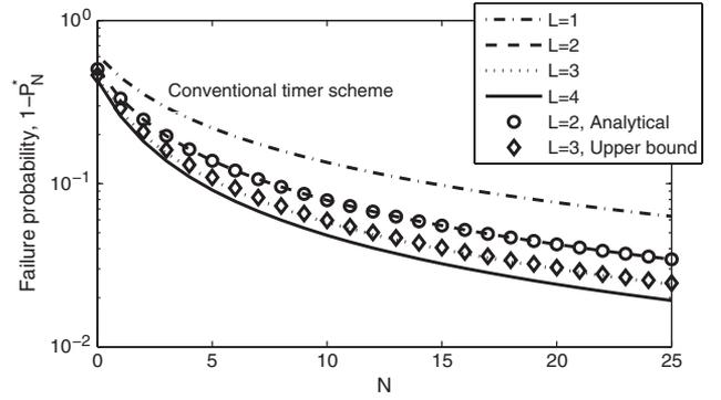
Fig. 2. Failure probability  $1 - P_N^*$  for different number of power levels and  $N$  ( $K = 10$  and  $\eta = 1$ ).
