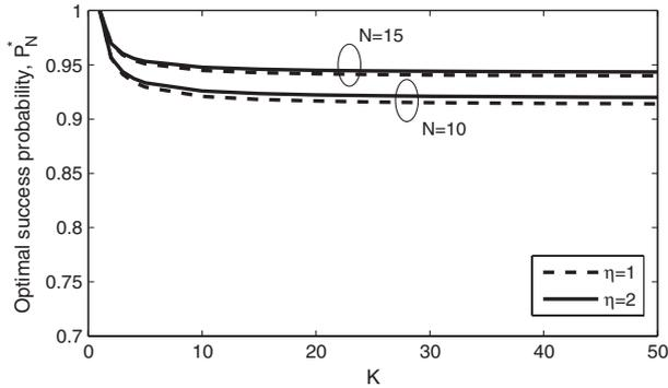
Fig. 4. Scalability evaluation: Zoomed-in view of optimal success probability  $P_N^*$  as a function of the number of nodes  $K$  for different  $\eta$  ( $L = 2$ ).
