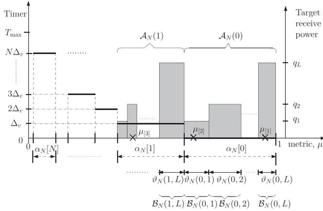
Fig. 1. Illustration of metric-to-timer-and-power mapping and how different metrics lead to different timers and target receive powers. The shaded vertical bars represent target receive power.
