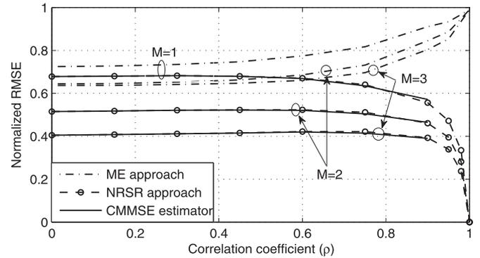
Fig. 2. Normalized RMSE ( $\text{RMSE}/(2\sigma^2)$ ) as a function of correlation coefficient  $\rho$  for different approaches ( $N = 10$  and  $\sigma^2 = 4.5$  dB).
