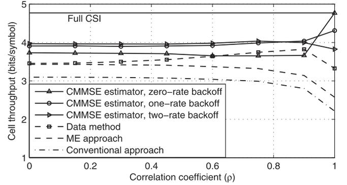
Fig. 7. PF scheduler for  $M = 1$  with statistically non-identical users: Zoomed-in view of cell throughput as a function of correlation coefficient  $\rho$  for different approaches ( $K = 10$ ,  $N = 10$ ,  $\alpha = 1.4$ , and  $\sigma^2 = 4.5$  dB).
