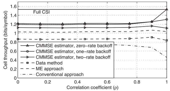
Fig. 5. RR scheduler for  $M = 3$  with statistically identical users: Cell throughput as a function of correlation coefficient  $\rho$  for different approaches ( $K = 10$ ,  $N = 10$ , and  $\sigma^2 = 4.5$  dB).
