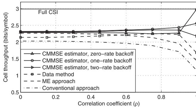
Fig. 3. Greedy scheduler for  $M = 1$  and statistically identical users: Zoomed-in view of cell throughput as a function of correlation coefficient  $\rho$  for different approaches ( $K = 10$ ,  $N = 10$ , and  $\sigma^2 = 4.5$  dB).
