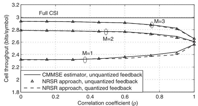
Fig. 6. Greedy scheduler with statistically identical users: Zoomed-in view of cell throughput as a function of  $\rho$  for unquantized SNR feedback and quantized feedback from users ( $K = 10$ ,  $N = 10$ , and  $\sigma^2 = 4.5$  dB).
