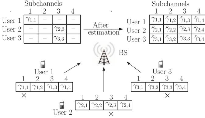
Fig. 1. Illustration of best- $M$  feedback by  $K = 3$  users and estimation at the BS ( $N = 4$  and  $M = 1$ ). Cross marks ( $\times$ ) denote the subchannels that are fed back.
