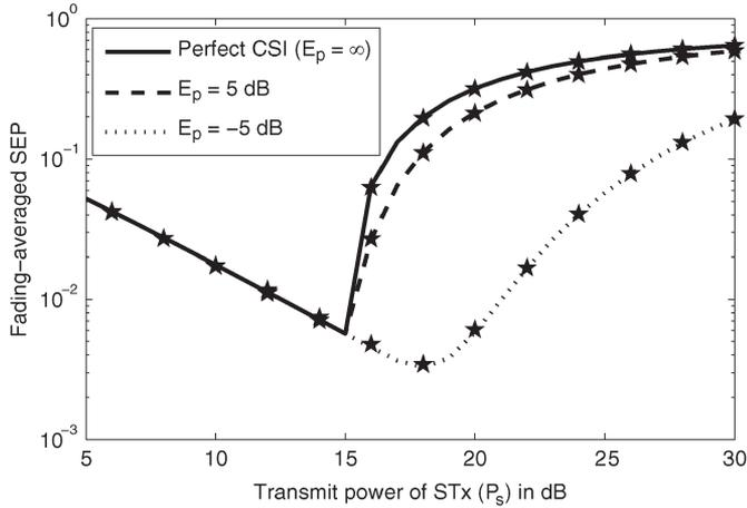
Fig. 3. Impact of imperfect CSI and transmit power of STx on the SEP of an average interference constrained SU ( $I_{th} = 15$  dB, QPSK, and  $N = 2$ ). Simulation results are shown using  $\star$  and analytical results using lines.
