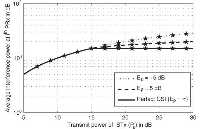
Fig. 2. Impact of imperfect CSI and transmit power of STx on the average interference at the  $i^{\text{th}}$  PRx ( $I_{\text{th}} = 15$  dB and  $N = 2$ ). Simulation results are shown using  $\star$  and analytical results using lines.
