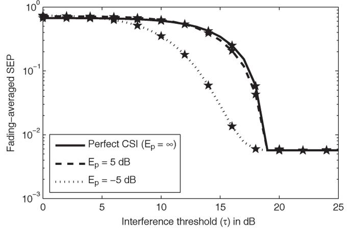
Fig. 5. Impact of imperfect CSI and interference threshold on the SEP of an interference outage probability constrained SU ( $P_{out} = 0.1$ ,  $P_s = 15$  dB, QPSK, and  $N = 2$ ). Simulation results are shown using  $\star$  and analytical results using lines.
