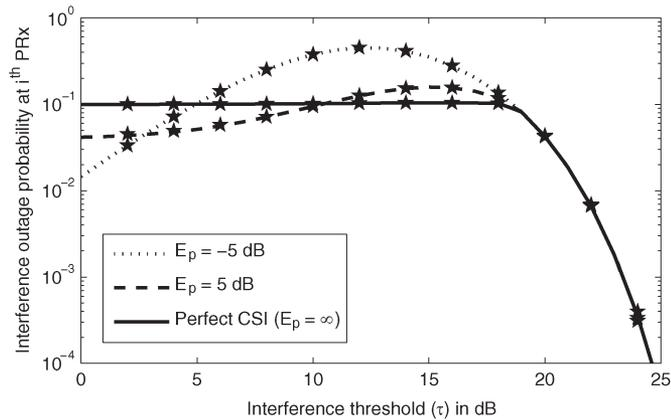
Fig. 4. Impact of imperfect CSI and interference threshold on the interference outage probability at each PRX ( $P_{out} = 0.1$ ,  $P_s = 15$  dB, and  $N = 2$ ). Simulation results are shown using  $\star$  and analytical results using lines.
