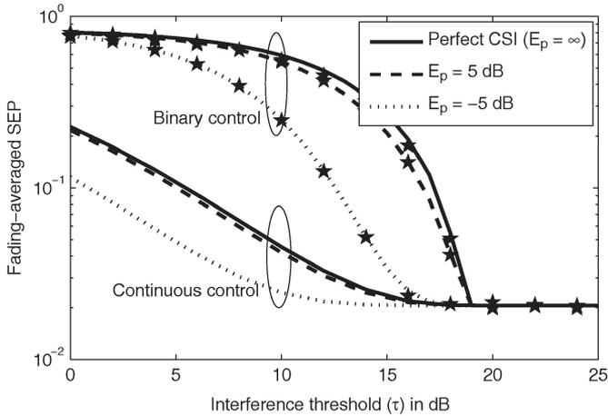
Fig. 7. Impact of binary and continuous transmit power constraints on the SEP of an interference outage probability constrained CR ( $\sigma_g^2 = 1$ ,  $\sigma_h^2 = 5$ ,  $P_{\text{out}} = 0.1$ ,  $P_s = 15$  dB, 8PSK, and  $N = 1$ ). Simulation results are shown using lines and analytical results using  $\star$ .
