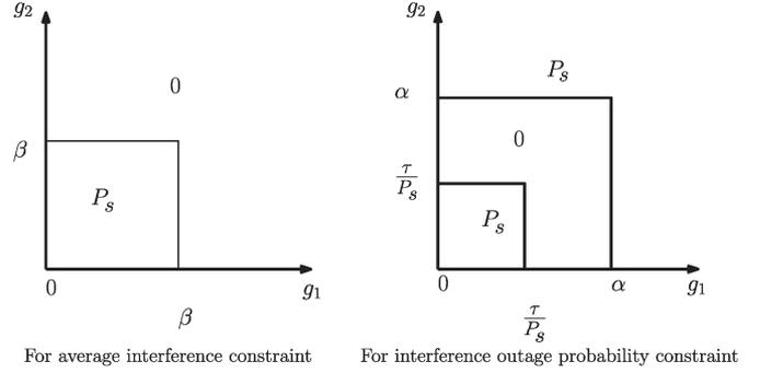
Fig. 1. Structure of optimal BPC policies ( $N = 2$ ).
