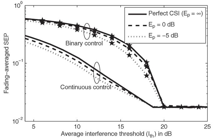
Fig. 6. Impact of binary and continuous transmit power constraints on the SEP of an average interference constrained CR ( $\sigma_g^2 = 10$ ,  $\sigma_h^2 = 5$ ,  $P_s = 10$  dB, QPSK, and  $N = 1$ ). Simulation results are shown using lines and analytical results using  $\star$ .
