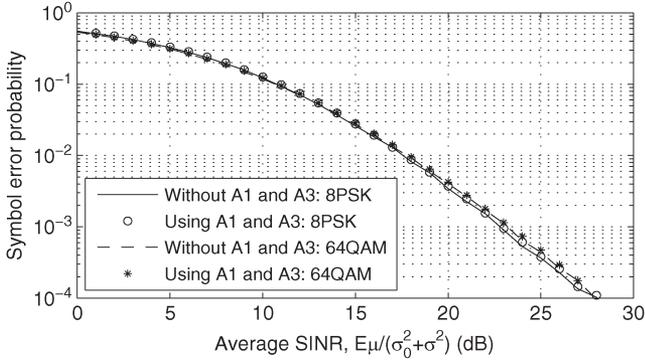
Fig. 1. SEP as a function of average SINR when the primary interference is approximated as Gaussian and  $T$  transmits 8PSK and 64QAM symbols ( $E_s = E_r = E = 10$  dB,  $\sigma_1^2 = \sigma_2^2 = \sigma^2 = 1.98$  dB,  $\sigma_0^2 = 2$  dB, and mean channel power gains of SD, SR, RD, and RX links are  $\mu$ ).
