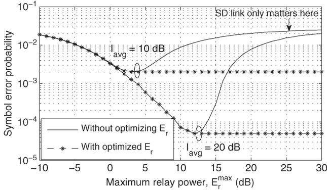
Fig. 5. IOA rule: SEP as a function of maximum relay power and  $I_{avg}$ , with and without optimizing  $E_r$  (QPSK,  $E_s = 10$  dB,  $L = 4$ , and  $\mu = 10$  dB).
