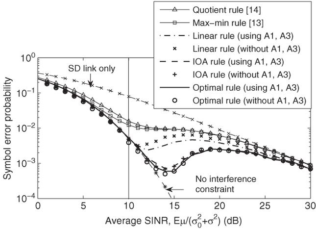
Fig. 2. Comparison of the SEPs of the optimal, IOA, linear, quotient, and max-min rules (QPSK,  $L = 4$ , and  $I_{\text{avg}} = 15$  dB).
