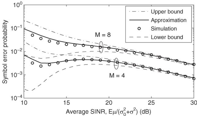
Fig. 6. *Linear rule*: SEP as a function of average SINR for different constellation sizes ( $L = 4$ ,  $I_{avg} = 15$  dB, and  $E_s = E_r = E = 10$  dB).
