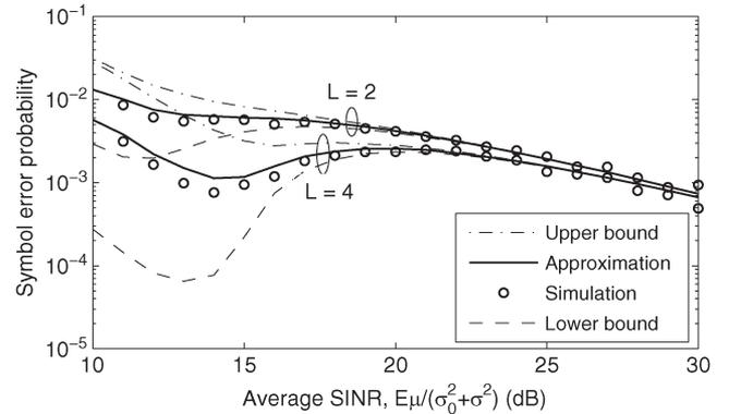
Fig. 4. *IOA rule*: SEP as a function of average SINR for different number of relays (QPSK,  $I_{\text{avg}} = 15$  dB,  $\mu_{SD} = \mu_{RX} = \mu$ ,  $\mu_{SR} = 0.75\mu$ , and  $\mu_{RD} = 1.25\mu$ ).
