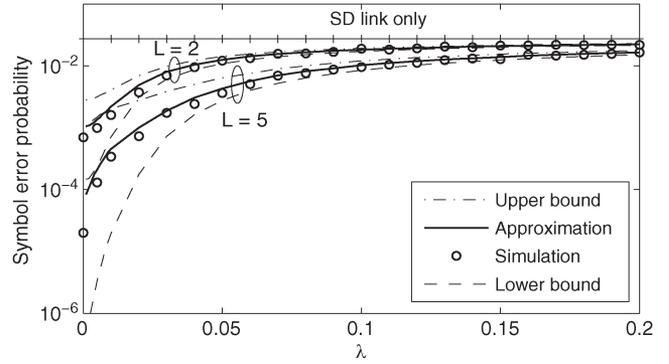
Fig. 3. Effect of  $\lambda$  on SEP of the IOA rule: SEP as a function of  $\lambda$  for two different values of  $L$  (QPSK and average SINR of 15 dB).
