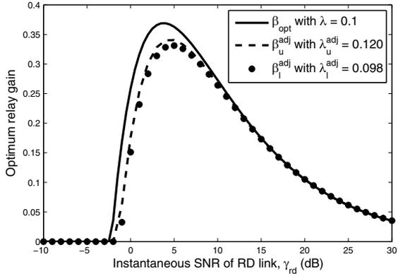
Fig. 3. Comparison of  $\beta_{\text{opt}}$ ,  $\beta_u^{\text{adj}}$ , and  $\beta_l^{\text{adj}}$  as a function of the instantaneous RD link SNR,  $\gamma_{rd}$  ( $\gamma_{sr} = 0.5$  dB,  $\lambda = 0.1$ , and QPSK).
