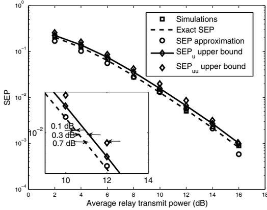
Fig. 4. SEP and its bounds as a function of average relay transmit power,  $\bar{P}_r$  ( $\bar{\gamma}_{sr} = \bar{\gamma}_{rd} = \bar{\gamma}_{sd} = P_s$ ,  $P_s = \bar{P}_r$ , and QPSK).
