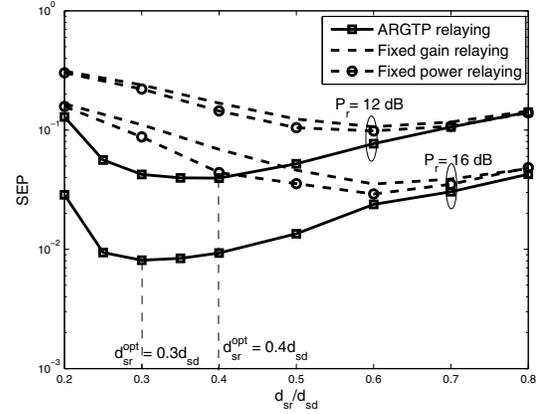
Fig. 9. Optimal relay placement: SEP of ARGTP relaying, fixed gain relaying, and fixed power relaying as a function of  $d_{sr}$  ( $P_s = \bar{P}_r$ ,  $\eta = 4$ , and QPSK).
