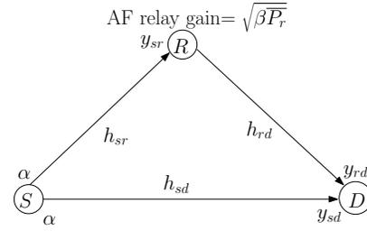
Fig. 1. Average relay transmit power constrained and variable gain AF relay model
