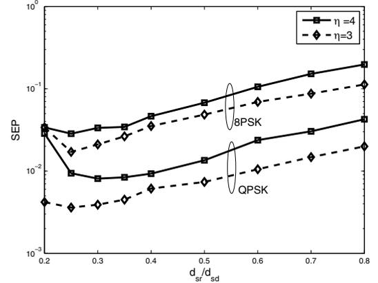
Fig. 10. Optimal relay placement: SEP of ARGTP relaying as a function of  $d_{sr}$  ( $P_s = \bar{P}_r = 16$  dB).
