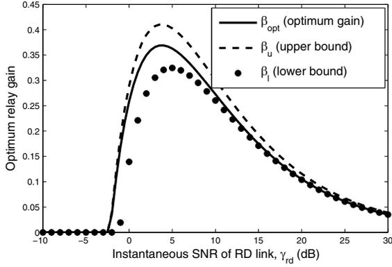
Fig. 2. Comparison of optimum relay gain,  $\beta_{\text{opt}}$ , its upper bound,  $\beta_u$ , and its lower bound,  $\beta_l$ , as a function of the instantaneous RD link SNR,  $\gamma_{rd}$  ( $\gamma_{sr} = 0.5$  dB,  $\lambda = 0.1$ , and QPSK).
