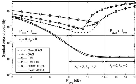
Fig. 6. MPSK: Comparison of the SEPs of CBBOASPA with Exact ASPA and benchmark policies ( $N_t = 2$ ,  $N_r = 1$ ,  $I_{ave} = 8$  dB, and BPSK).
