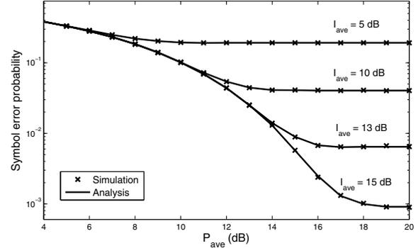
Fig. 3. SEP as a function of  $P_{\text{ave}}$  for different values of  $I_{\text{ave}}$  ( $N_t = 2$ ,  $N_r = 1$ , and 8PSK).
