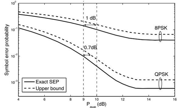
Fig. 4. SEP and its upper bound as a function of  $P_{\text{ave}}$  for different constellation sizes ( $I_{\text{ave}} = 10$  dB,  $N_t = 2$ , and  $N_r = 1$ ).
