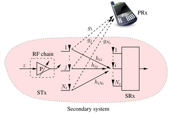
Fig. 1. System model with one PRx and a secondary system consisting of an STx with  $N_t$  transmit antennas and one RF chain that communicates with an SRx with  $N_r$  receive antennas.
