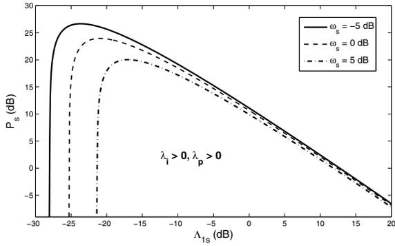
Fig. 2. Transmit power from selected antenna in the power- cum interference-constrained regime ( $I_{\text{ave}} = 10$  dB,  $\bar{\omega} = 1$ ,  $\bar{\Lambda} = 1$ ,  $\sigma^2 = 1$ , and  $P_{\text{ave}} = 12$  dB).
