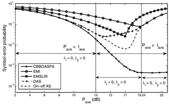
Fig. 7. MQAM: Comparison of the SEPs of CBBOASPA and benchmark policies ( $N_t = 4$ ,  $N_r = 1$ ,  $I_{ave} = 13$  dB, and 16QAM).
