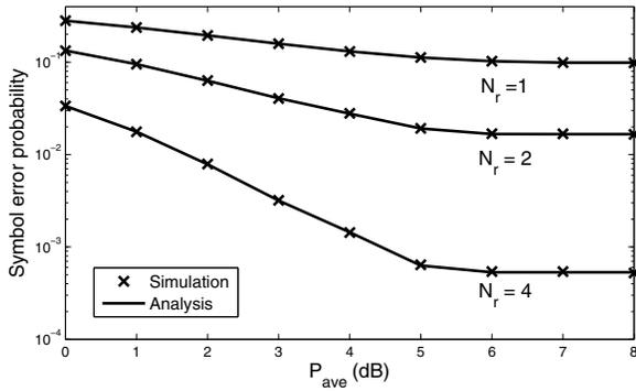
Fig. 5. Effect of number of receive antennas: SEP as a function of  $P_{\text{ave}}$  for different  $N_r$  ( $I_{\text{ave}} = 2$  dB,  $N_t = 2$ , and QPSK).
