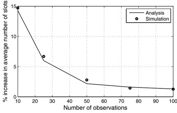
Fig. 6. Percentage increase in the average time required to select the best relay as a function of the number of observations used to estimate the CDF. Parametric estimation is used and the metrics are exponentially distributed RVs with unit mean ( $\zeta = 1$  and  $n = 10$ ).
