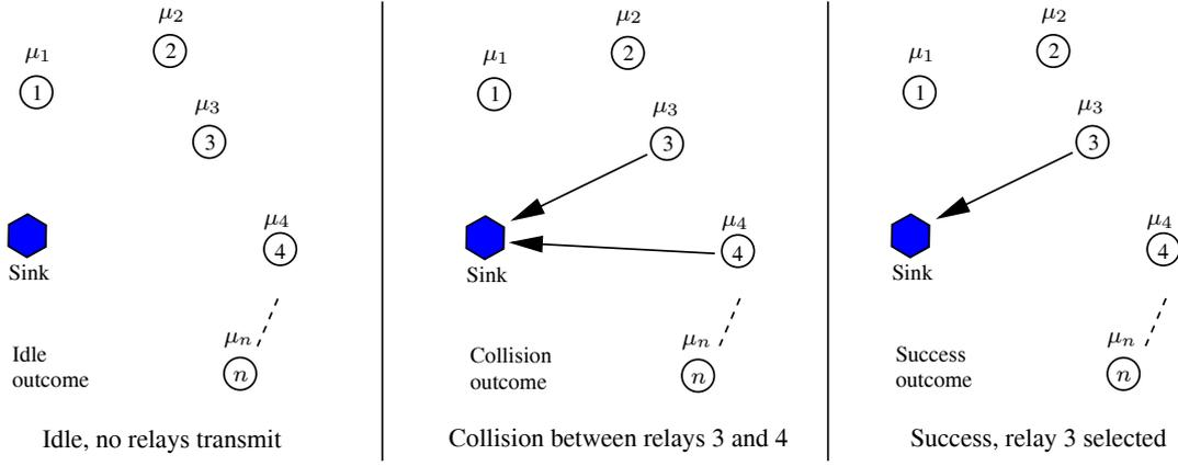
Fig. 1. A system consisting of a sink and  $n$  relays, in which the metric of relay  $i$  is  $\mu_i$ . The figure illustrates how the  $n$  relays contend in the splitting based selection algorithm, how the three scenarios of idle, success, and collision arise over a duration of three slots, and how the relay with the highest metric gets selected.
