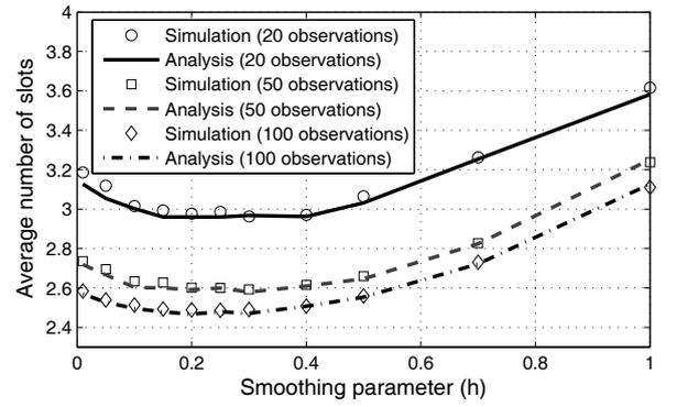
Fig. 7. Zoomed-in view of the average number of slots required to select the best relay as a function of the smoothing parameter  $h$  used for non-parametric estimation. Gaussian kernel estimator is used and the metrics are exponentially distributed random variables with unit mean ( $\zeta = 1$  and  $n = 10$ ).
