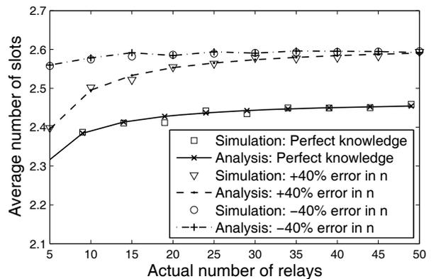
Fig. 5. Zoomed-in view of the average number of slots required to select the best relay when the assumed number of relays is incorrect ( $\zeta = 1$ ). A ‘+40% error in  $n$ ’ means  $n_{\text{asm}} = 1.4n$ , while a ‘-40% error in  $n$ ’ means  $n_{\text{asm}} = 0.6n$ .
