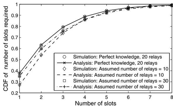
Fig. 4. CDF of the number of slots required to select the best relay when the assumed number of relays is incorrect ( $\zeta = 1$  and  $n = 20$ ).
