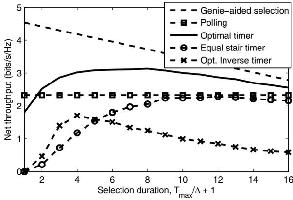
Fig. 6. Net throughput as a function of selection duration ( $K = 20$ ,  $p = 0.4$ , and  $T_c = 40\Delta$ ).
