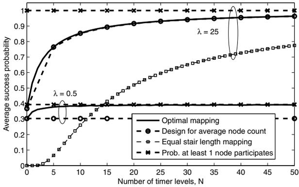
Fig. 4. Poisson prior: Benchmarking of average success probability as a function of the number of timer levels for optimal mapping, design for average node count, and equal stair length mapping for  $\lambda = 0.5$  and  $\lambda = 25$ .
