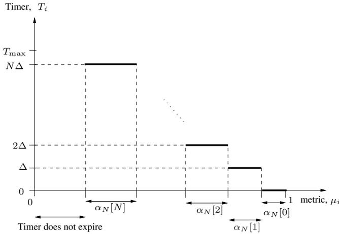
Fig. 1. Illustration of a staircase metric-to-timer mapping for a maximum selection duration of  $T_{\max}$  and a vulnerability window  $\Delta$ .
