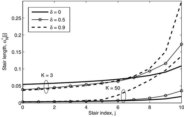
Fig. 7. Stair lengths of the robust mapping as a function of  $j$  for different uncertainties.
