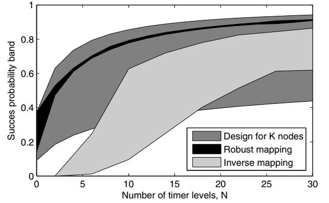
Fig. 8. Comparison of success probability bands as a function of the number of timer levels of the robust mapping, inverse mapping, and design for  $K$  nodes ( $K = 50$  and  $\delta = 0.9$ ).
